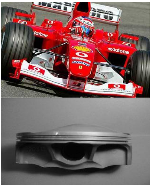
Fig.4. The Formula 1 racing car and its Al-alloy piston studied by SANS
